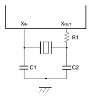
**Remark** For the resonator selection and oscillator constant, customers are requested to either evaluate the oscillation themselves or apply to the resonator manufacturer for evaluation.
